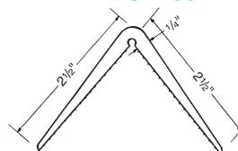
Koroseal Vinyl Corner Guards prevent corner damage from wheeled carts in hospitals and other commercial buildings. Abrasion-resistant vinyl has good wearing and rebounding qualities; is easy to clean. Standard 54" lengths. Install with #400 Contact Cement.
