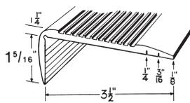
Ribbed Koroseal Vinyl butt-type nosing for front edge of stages, bowling lanes steps, platform-like floors and bar foot rests. Grooved cutting guides provide "cut-offs" to match flooring thickness. Standard 8' lengths; easily cut to size. Install with #400 Contact Cement.
