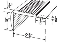
Ribbed Koroseal Vinyl lap-type nosing for front edge of stages, bowling lanes steps, platform-like floors and bar foot rests. Form fitting adjusta-nose; has a 7/8" lip to allow 1/8" flooring to lap over back edge. Standard 8' lengths. Install with #400 Contact Cement.
