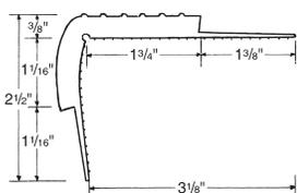
Improve safety and prevent worn carpet edges on steps. For new or renovation work. Butt 1/4" to 3/8" thick carpet against both the top and bottom lips of butt-type carpet nosing. Standard 8' lengths, easily cut to shorter lengths. Install with #400 Contact Cement.
