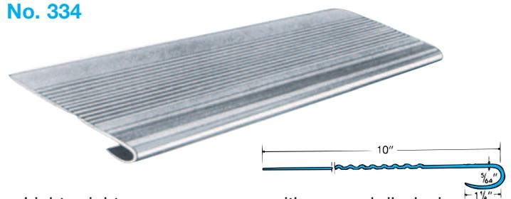
Lightweight, economy gauge with a round rib design. Wear and tear resistant Koroseal will give years of service; compares with heavier weight treads. Curve-around nose fits round or square nose steps. Intended for residential or light commercial use.
