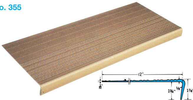
Lower cost production for multi-family dwellings, apartment houses, low income housing. This tread with extra long nose is designed to use on a 2" x 12" plank step or molded concrete step. Heavier thickness at front "wear area". Treads are easy to install; flat rib surface is easy to clean. Meets Fed. Specs. RR-T-650E Type B.
