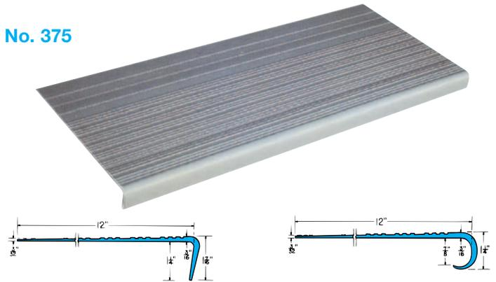
Designed for use in apartments, urban renewal housing, housing for the elderly and housing projects. Lower initial cost, ease of installation and cleaning, and long service appeals to owner and builder. Extra thick at front; Meets Fed. Specs. RR-T-650E Type B.
