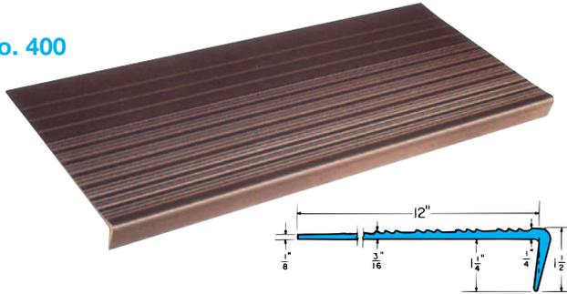
Heavy gauge sharp-rib design Koroseal vinyl tread for heaviest traffic; 1/4" thick at wear area, easily trimmed to cover and fit any stair step. Install over concrete, metal, wood, terrazzo. Extra heavy thickness at the front "wear area". Meets Fed. Specs. RR-T-650E Type B.
